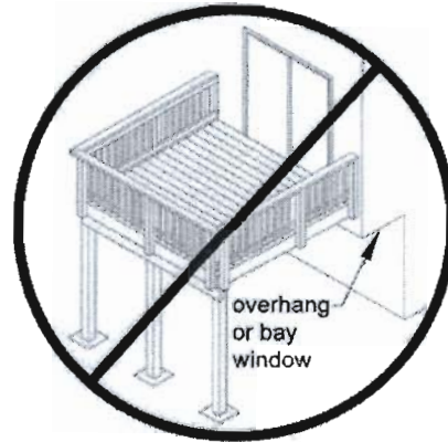
Figure 18: No Attachment to House Overhang
